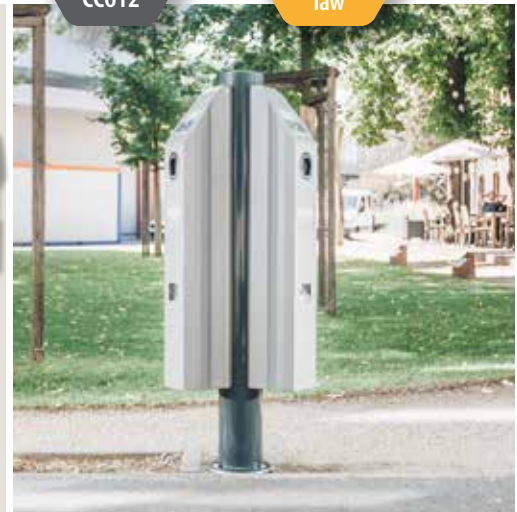
Figure 5: ebee's charging point Berlin (3.7 kW / 11 kW / 22 kW) from ebee has been designed for outdoor use (stainless steel, IP54, IK10, forced-ventilated). Installation is possible as a wall-box on a wall or by means of the optionally available pole as a free-standing single or double column. The poles can be mounted on suitable solid ground (concrete floors) or on loose soil or earth using the supplied ground anchor.
