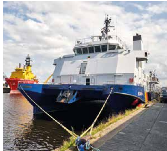
View of the double hull of the SWATH vessel Helgoland © Carsten Müller
